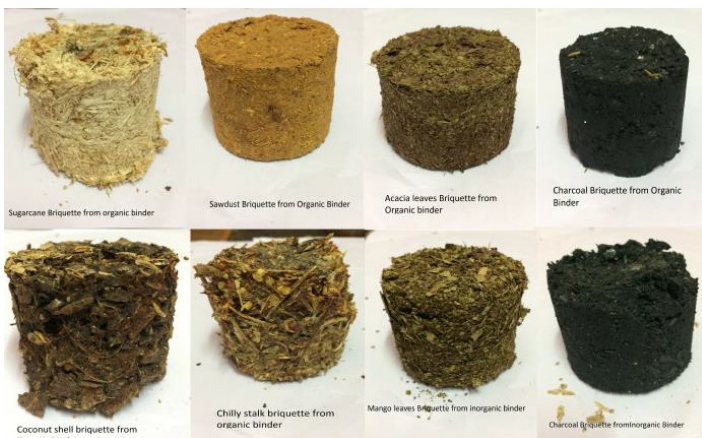
Fig.1 Showing briquettes made from organic and inorganic binder.
